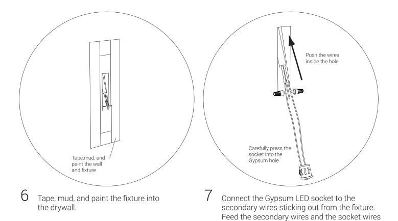
back into the hole in the Gypsum fixture.
